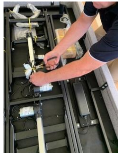
2. Cut zip ties Screw-In 4 feet
