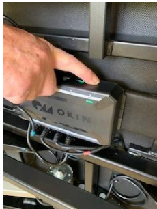
5. Pairing Press Remote Control PAIR button until blue light is flashing press control box PAIR button twice
