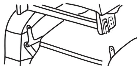
**4.1.2** Slide the left and right KD sleeves of the chair-back onto the KD connections on the arms and seat of the chair.
