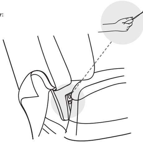
**4.3.2** Using a large flat-head screwdriver, lift the left and right locking clips on the chair-back one side at a time to raise the back from the connections on the chair base. As you lift each locking clip, pull up on the chair-back to lift that side over the lock.
