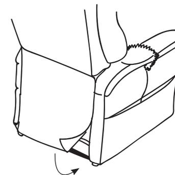
**4.1.4** Attach the chair-back to the hook and loop flaps on the bottom of the chair base.
