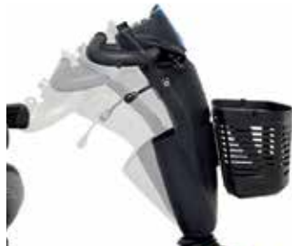
Users can easily adjust the tiller with a lever to suit their needs.
