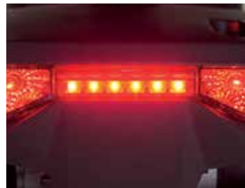
Clear, bright brake lighting warns people that the scooter is slowing down.
