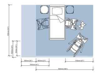
Blue area shows the minimum working area required to enable the caregiver to use the mechanical aids ergonomically from one side.
